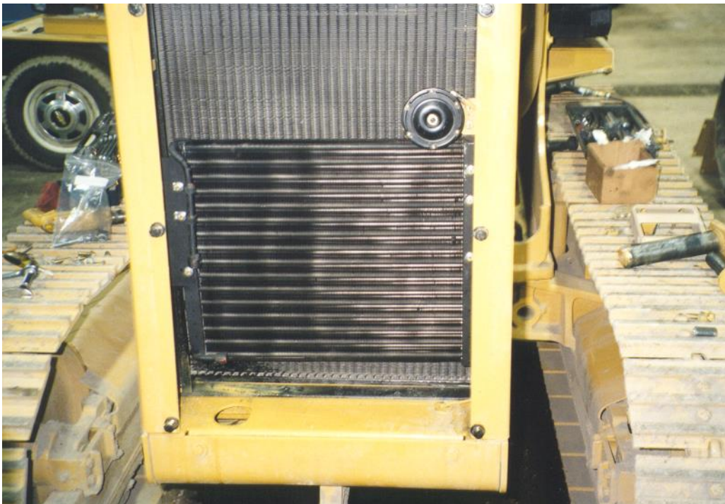
Condenser in place on radiator.
