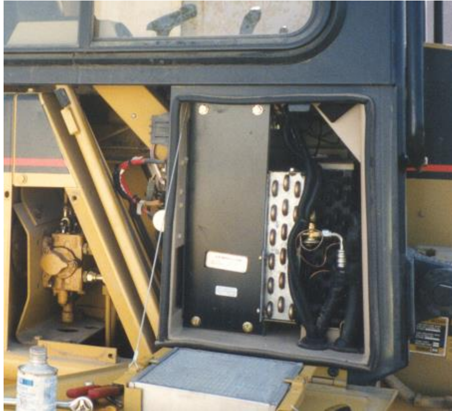
Evaporator assembly in place with lines run.
