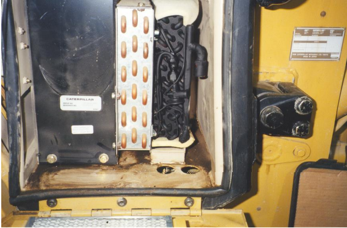
Evaporator in place against heater assembly.
